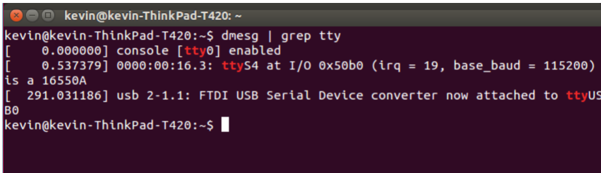
Figure 5. Determining the TTY device that corresponds to the UART-to-USB connection.
